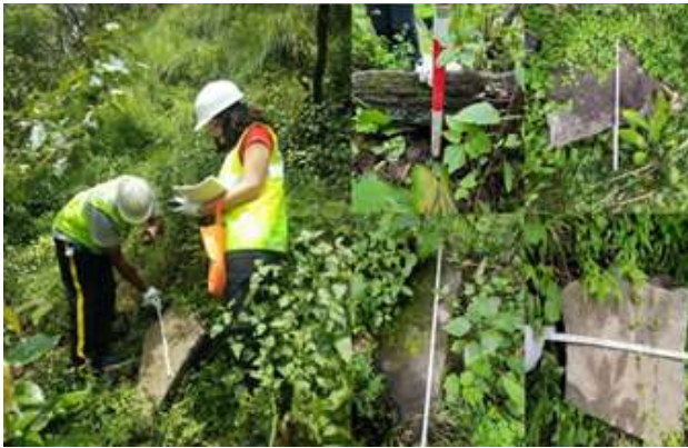
Figure 2, Rock boulders measurement carried out on the slope and deposition area.
