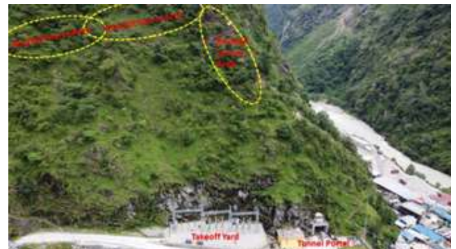
Figure 1, Drone image showing the rockfall deposition and source area including vulnerable area
