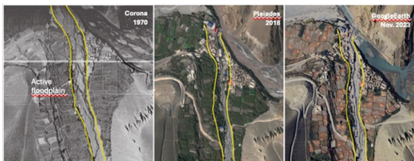
Figure 4, Evolution (1970–2023) of the Jhong Khola active floodplain at Kagbeni. Left (1970): an active floodplain with intermittent flows and gravel bars bounded by cultivated lower terraces. Middle (2018): settlement expansion into the former floodplain. Right (2023): the Jhong Khola reoccupied its natural flooding zone during the flood.
