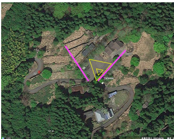
Figure 1, Survey site. TKSH06 is a seismic station. Triangle shows the array with 29m and 4m sizes.
