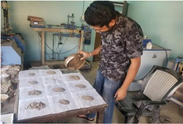
Figure 5, Showing the process of the sieve analysis.
