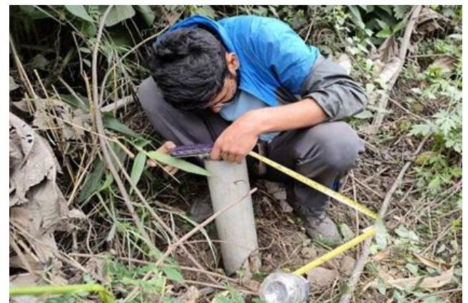
Figure 4, Process of infiltration test done at the study area.
