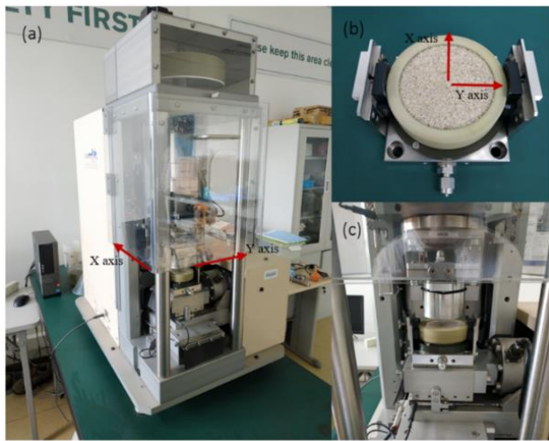
Figure 2, Simple shear apparatus used in this study: (a) VDDCSS; (b) specimen and axes definition; (c) specimen before consolidation.
