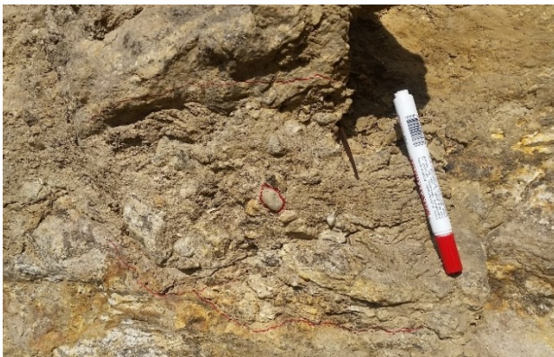
Figure 2, Sub-rounded pebbles present above 20 m uphill side from damsite area.
