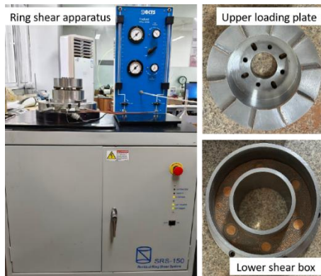
Figure 2, SRS-150 ring shear apparatus.
