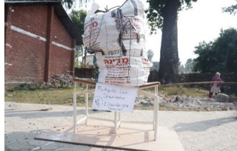
Figure 3, Drop demonstration of EQ desks.
