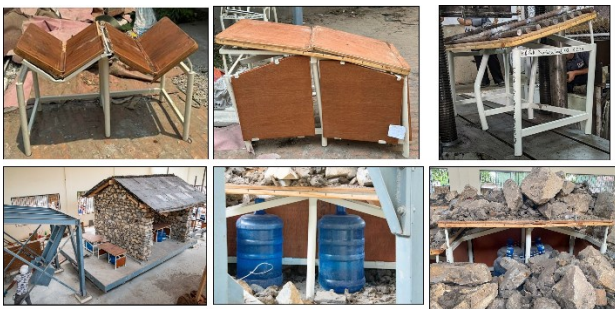
Figure 2, Vertical compression tests (top) and shock table test (bottom) of the EQ Desks.
