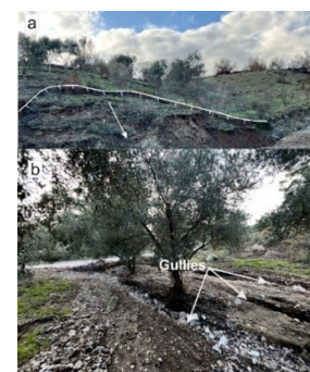
Figure 1, In the aftermath of wildfires a) shallow failures b) gullies filled with debris in the lower catchment.
