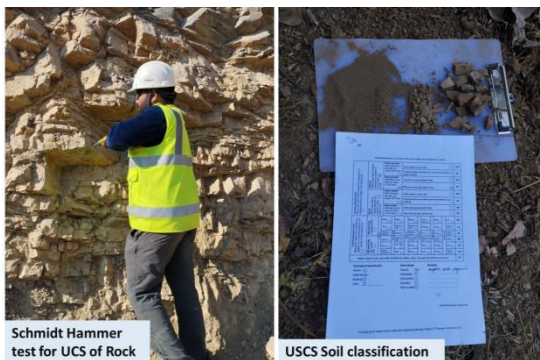
Figure 2, Field investigation activities including Schmidt hammer testing and in-situ USCS soil classification.
