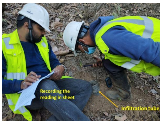
Figure 3, Infiltration assessment at Jamunedanda using the inverse-borehole method.
