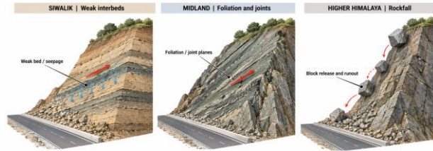
Figure 2. Conceptual failure mechanisms commonly encountered in landslide and road cuts: weak interbeds, structurally controlled movement along foliation/joints, and rockfall.
