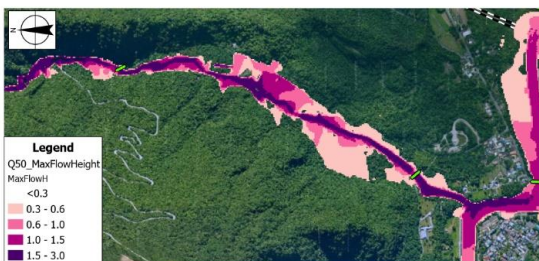
Figure 3, Max flow height during debris flow simulation in Q50 scenario.
