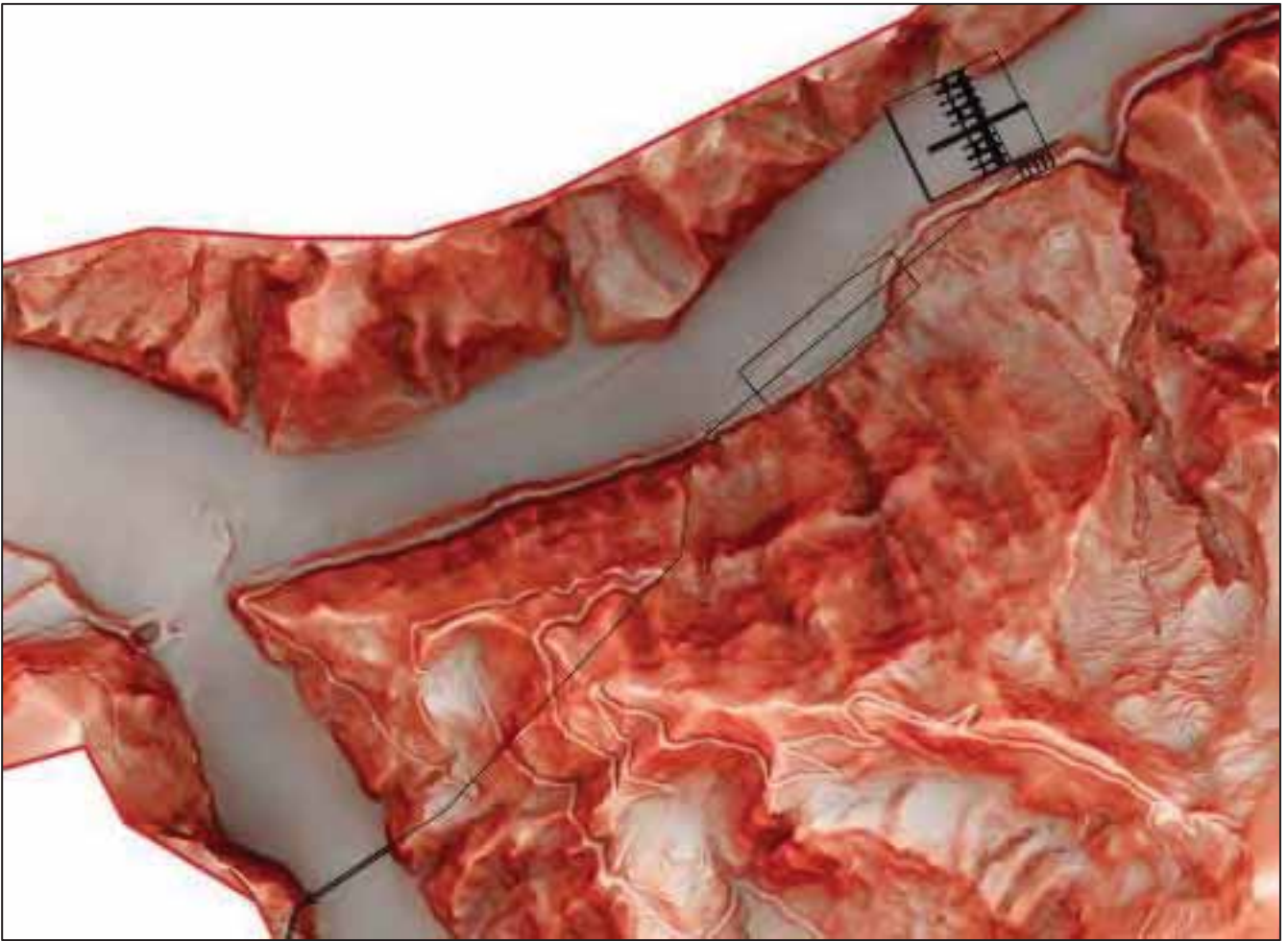
Figure 12, Example of a RRIM generated from LiDAR survey data.
