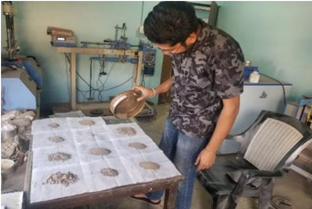
Figure 5, Showing the process of the sieve analysis.
