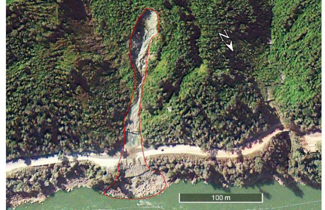
Figure 11, Satellite image of debris flow at Simaltal triggered by 2010 rainfall from GoogleEarth (2010/11/02).
